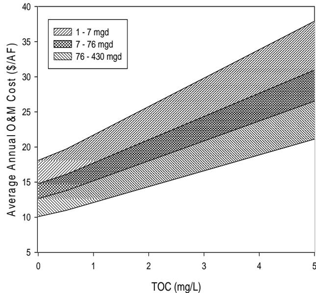
Figure 4. Effects of total organic carbon concentration on annual operation and maintenance cost of enhanced coagulation. The cost result shown in the figure was estimated by author's calculation using EPA (USEPA 2005) and MWDSC (Lu et al. 2007). The costs were converted to 2007 dollars using deflators from ENR and BLS.
