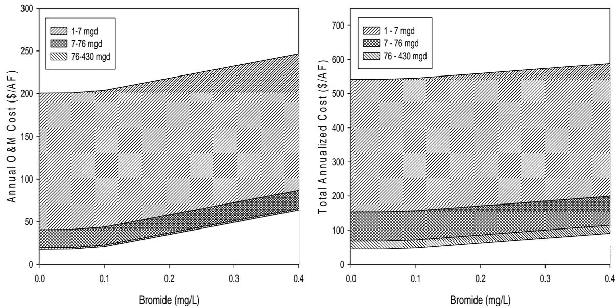
Figure 3. Bromide concentration effects on total annualized cost and annual O&M cost of ozonation for disinfection and oxidation in conventional water treatment. The cost results shown in the figure were estimated by authors' calculations using EPA (USEPA 1999; USEPA 2005) and MWDSC (Krasner et al. 2007; Lu et al. 2007). The costs were converted to 2007 dollars using deflators from ENR and BLS.
