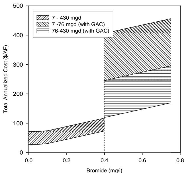
Figure 5. Effects of bromide concentration on annual O&M cost of enhanced coagulation and ozonation in combination with granular activated carbon added above  $0.4 \text{ g l}^{-1}$ . The cost result shown in the figure was calculated using the cost data from Figure 3 and 4 and Table 4.
