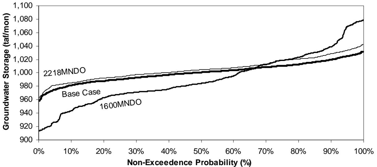
**Figure F.18 - Statewide groundwater storage non-exceedence for increasing minimum net Delta outflow**
