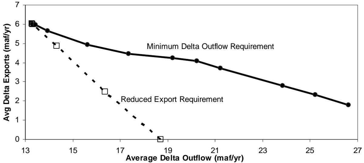
**Figure F.S1 - Average Delta exports for a given level of Delta outflow for the two regulatory alternatives (reduced exports and increased minimum net Delta outflow)**
