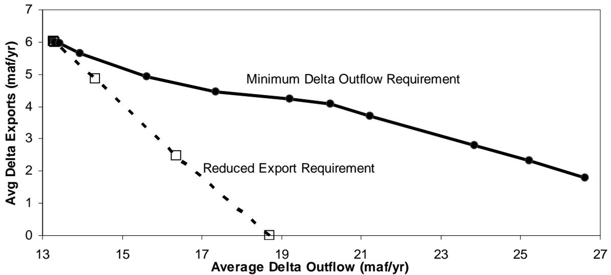
**Figure F.19 - Average Delta exports for a given level for Delta outflow for the two alternatives (reduced export capacity and increased minimum net Delta outflow)**
